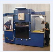
Maximum Control of Hazardous Dust Wet collector, plus containment enclosure, plus regain-air plenum.
