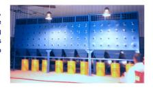
BOB. The Blow-Off Booth provides workers a powerful cleaning station as they leave the dusty plant environment, increasing both worker comfort and contaminant control. The Blow-Off Booth is often used in places where the dust is carcinogenic.
