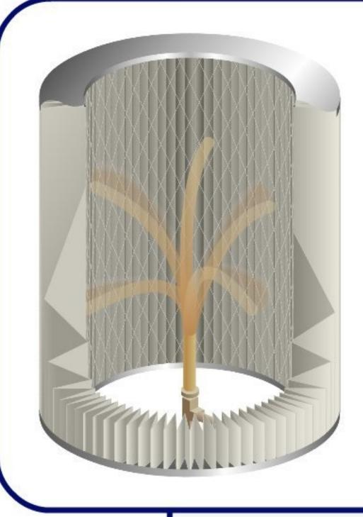
As compressed air reaches near-sonic velocity exiting from our Sonic Resonating Rapper<sup>TM</sup>, its whipping motion raps the inside of the cartridge, dislodging even the material deeply packed into the pleats, and returning the cartridge to start-up flow capacity.
